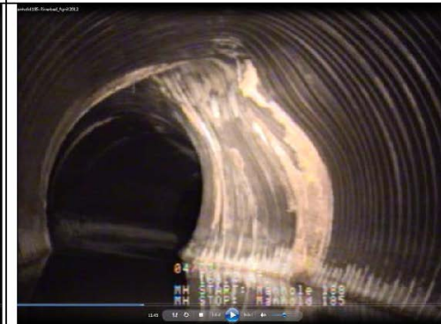
31: Deformation at the Bend Sta. 5 + 31.40 – 4/23/12
